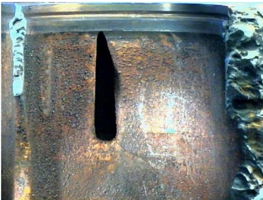
A 2 Cracked cylinder liner
