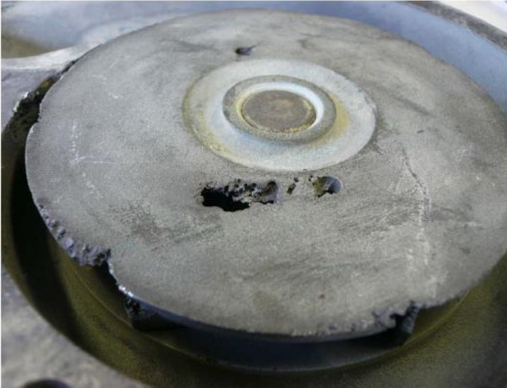
A 7 Flywheel of the coolant pump, cavitated
