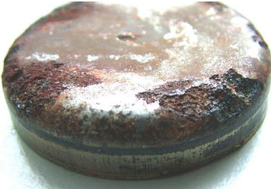
A 3 Sealing cover, corroded
