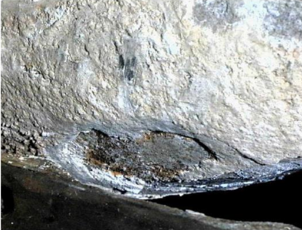
A 5 Limescale deposits on a cylinder liner
